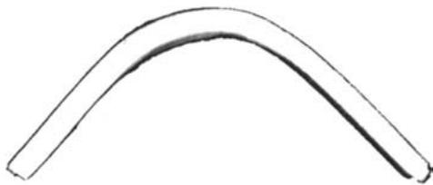
Figure 10 Bending test of the FSW weld.
